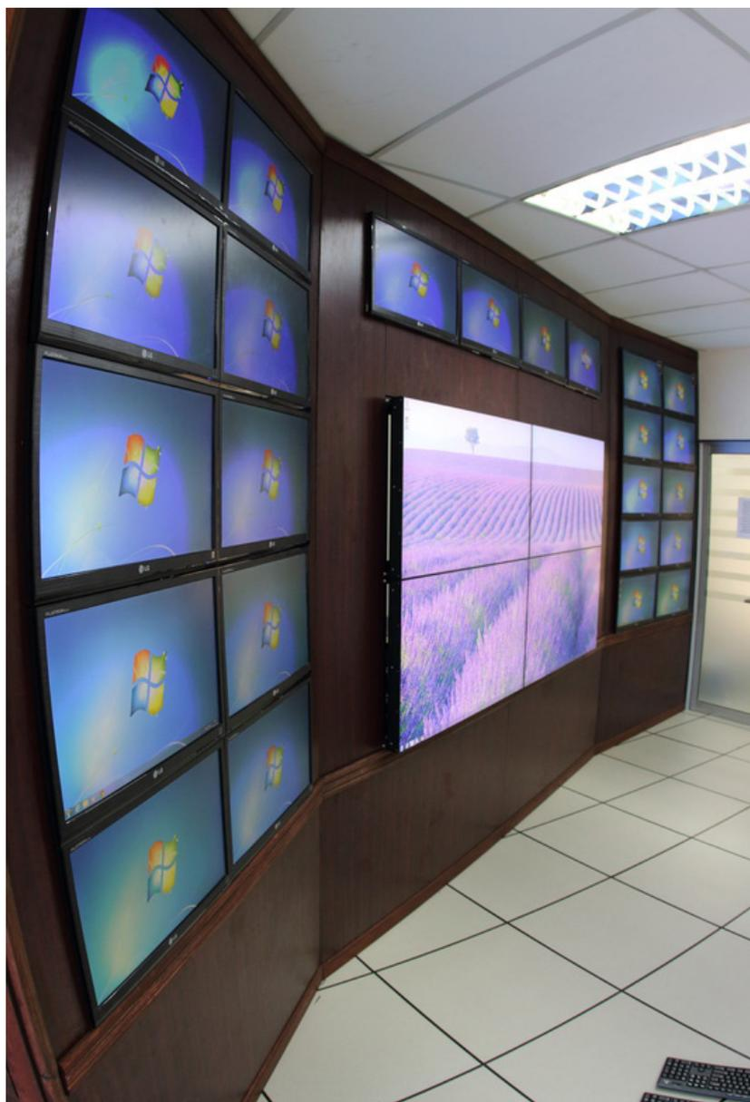
Three servers are used to cater for the 28 screen display. The system also deploys Datapath ImageDP4 graphics cards and VisionHD4 capture card technology, with seven ImageDP4 and four VisionHD4 units used on the project.
